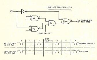
Fig. 3. Logic state relationships of the control signal implementation.
